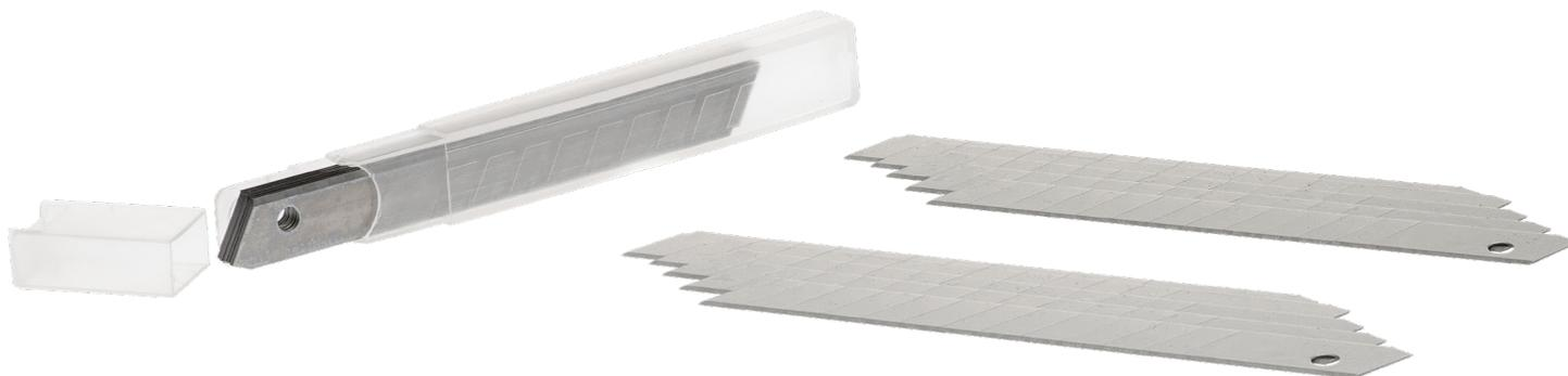
The KB004-10 is a 9mm Snap Blade made of SK-5 Japanese Steel. The blades are packed in a tube of 10 blades. These blades are universal and can fit in most other 9mm retractable knives on the market.
